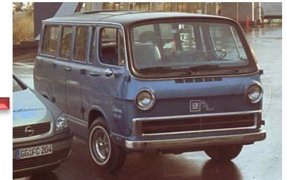
1967 – GM Electrován \text{LH}_2 , FC, 200 km range 105 km/h top speed
