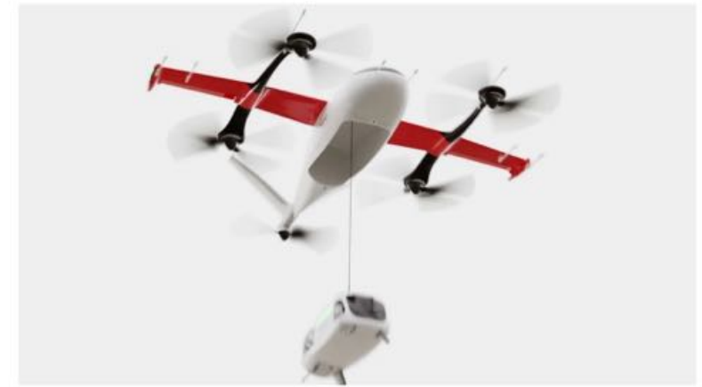
Zipline's drone delivery aircraft use a cable to lower this delivery device, called a droid, to deliver packages onto a precise spot. Zipline
